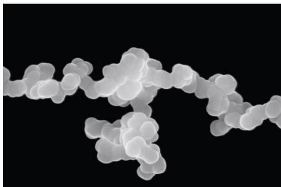
Figure 1b: Scanning electron microscope view of a typical carbon Black aggregate consisting of fused primary particles (magnification: x 120,000)
